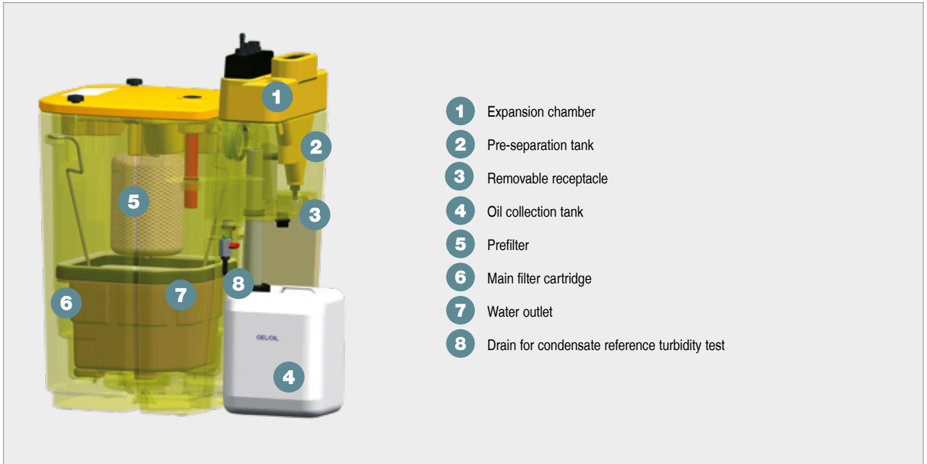
Fig. 3: Condensate separation system for compressed air using the gravity principle (functional diagram)
