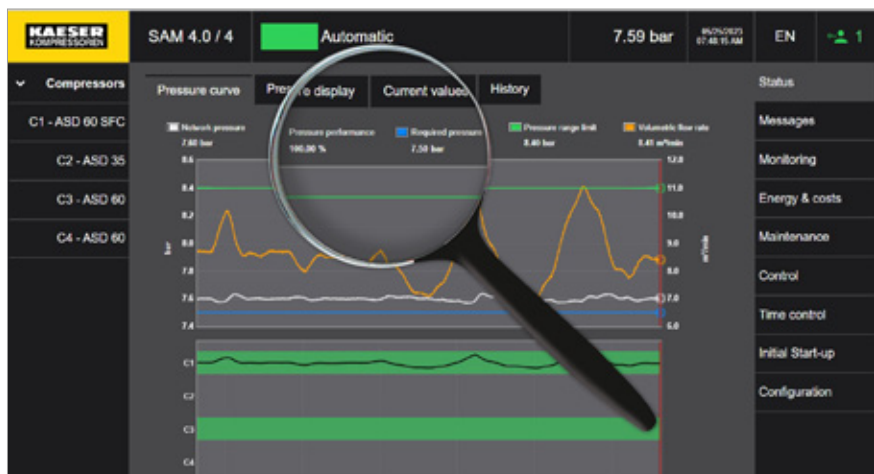
Fig. 5b: Flow rate and pressure curve with pressure performance monitoring
