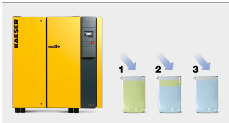
Fig. 2: Every compressor draws in water vapour and contaminants along with atmospheric air. The condensate resulting from compression (Fig. 2 (1)) must be free from oil and other harmful substances (Fig. 2 (2)) before it can be disposed of as normal wastewater (Fig. 2 (3)).
